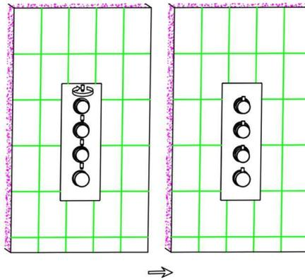
10. Screw the handles into the handwheels.
