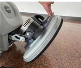
3. Install the burnishing pad on pad driver and Secure pad with center-lock. Do not operate machine without pad center-lock installed.
