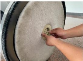
4. Pull the head lock knob to release the head from the pad change position.
