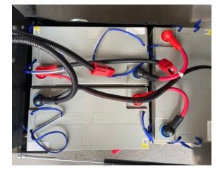
The machine is powered by a 36V battery pack. The burnishing process is accomplished by a high-speed rotating pad with applied pressure and forward motion creating a smooth polished floor finish. The pad pressure can be adjusted for floor type and floor condition. The pad pressure is mechanically adjusted. The burnishing function is controlled by a start bail at the control console.
